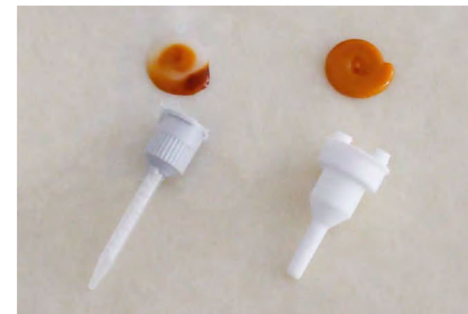
Comparison: Mixing result static mixing (left), mixing result dynamic mixing (right)
